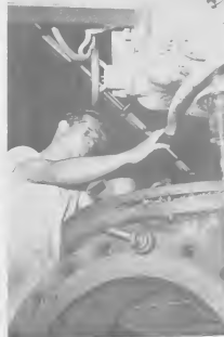
DRILLING COVER of a water strainer for the power N. Panneflek. The machine tool is a Carlton push-button automatic drill press.
